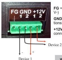
**FG** = Frame Ground (Do Not Connect to V-)
