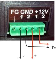
**FG** = Frame Ground (Do Not Connect to V-)
