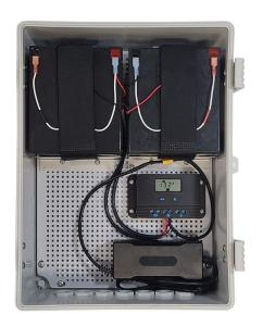
Attach the included battery cable to the controller BAT inputs. (Red to + and Black to –).
