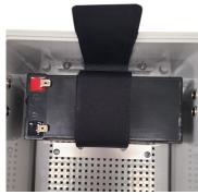
Fold the end of the strap between the battery and the enclosure wall to allow access to the end of the Velcro strap for easy removal.
