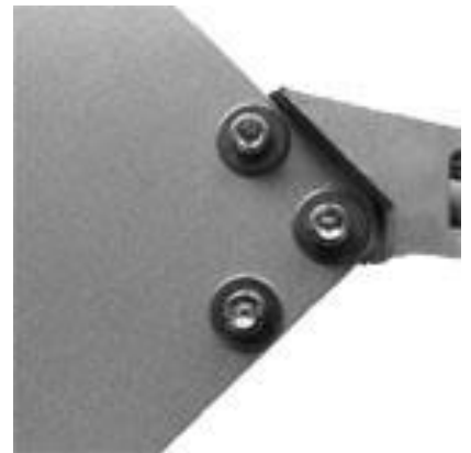
Figure 7.3: Fix the Tail Vane
