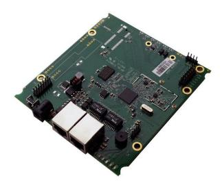
The EZ2+V3 is a high capacity 100Mbps and high power 300mW outdoor wireless bridge system operating in the 2.4GHz unlicensed spectrum.
