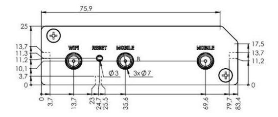
The figure below depicts an approximation of the device's dimensions when cables and antennas are attached:
