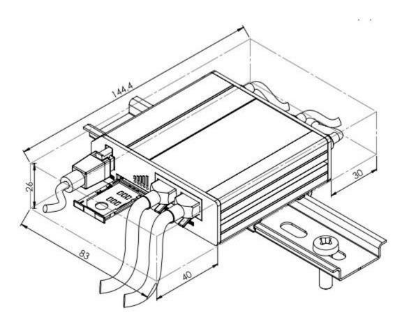
The scheme below depicts protrusion measurements of an attached DIN Rail:
