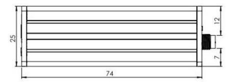
The figure below depicts the measurements of RUT241 and its components as seen from the front panel side:
